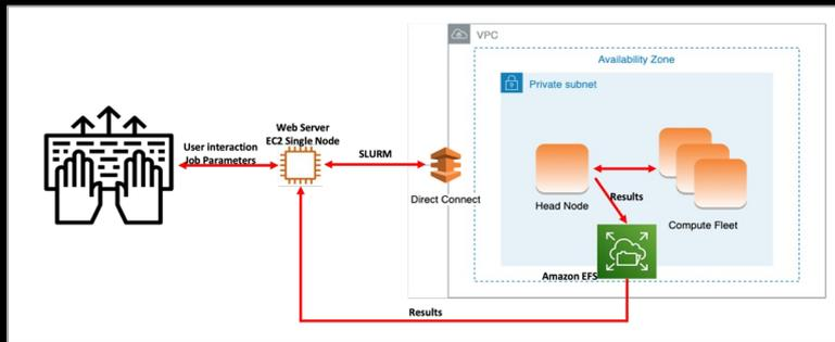
Left: Configuration of AWS platform. User interface is hosted on the single node instance and communicates with computing instance through SLURM scheduler. Computing instance is in isolated virtual private cloud (VPC) for higher security. Model results are stored in AWS elastic file system (EFS).
