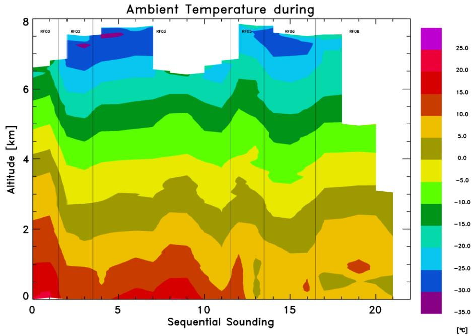
Figure 7: Color contours for all temperature measurements. All soundings are shown in the sequence in which they were released. White areas reflect the different release altitudes. The different science flights are separated by vertical lines and indicated near the top.
