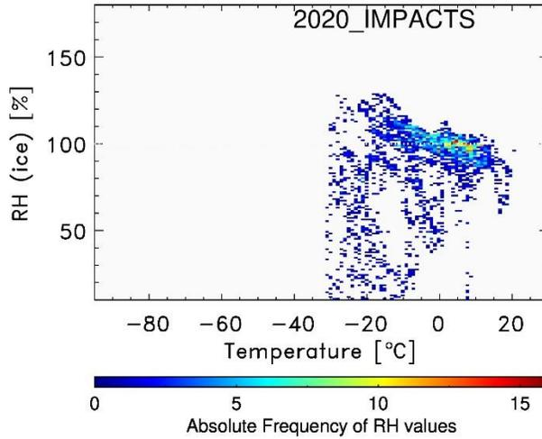
Figure 5: Density plots showing the correlation between all temperature and relative humidity measurements based on raw data. The color coding indicates the how often the combination of temperature and relative humidity was observed in the entire data set.
