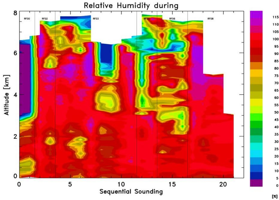
Figure 8: Color contours for all relative humidity measurements. Note that at temperatures below freezing, relative humidity is calculated with respect to ice.
