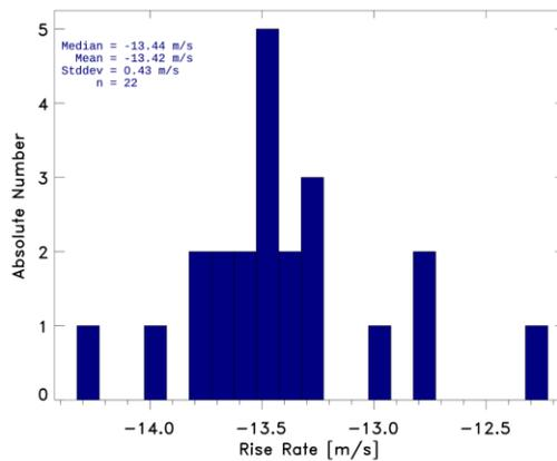
Figure 6: Median fall speed across the profiles for all dropsondes.
