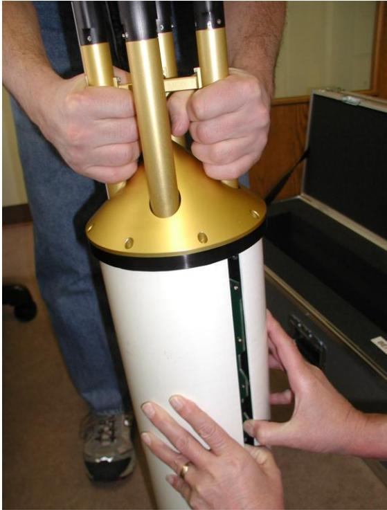
Figure C. Prying tube open at seam
