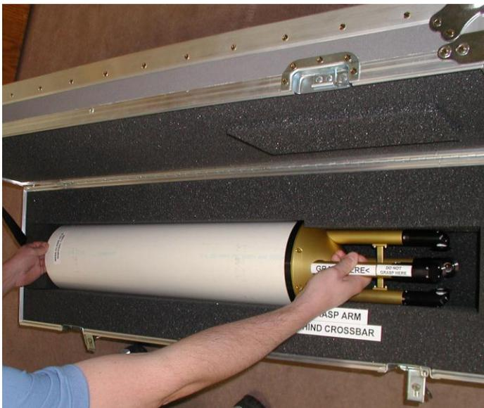
Figure A. Proper placement of hands on probe
