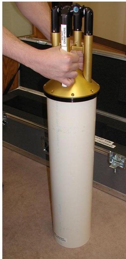
Figure B. Place Probe on Floor
