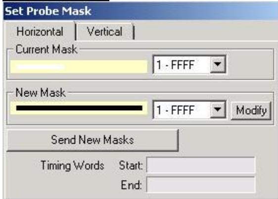
This window allows the operator to view the current mask on each array to see which elements are being masked out. This window should not be used to send new masks though it has that option, the Command Window is where the operator should request to build new masks while sending command packets to the probe.
