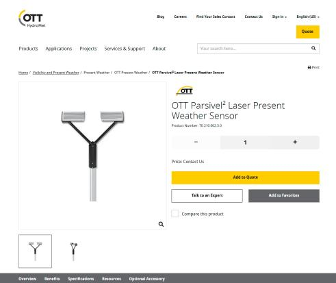
The OTT Parsivel² is a modern laser disdrometer for comprehensive measurement of all precipitation types. The Parsivel² captures both the size and speed of falling particles, classifying them into one of 32 separate size and velocity classes. The raw data are used to calculate the type, amount, intensity and kinetic energy of the precipitation, the visibility in the precipitation, and the equivalent radar reflectivity
