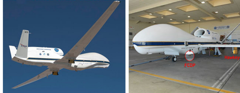
NASA Global Hawkeye UAV flies to altitudes of 65,000 ft and has a duration of 30 hours
