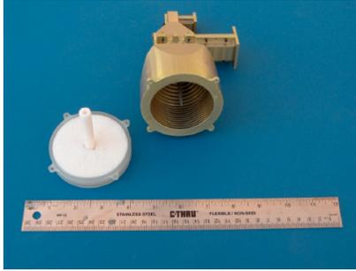
Fig. 3. Dual-frequency feed.
