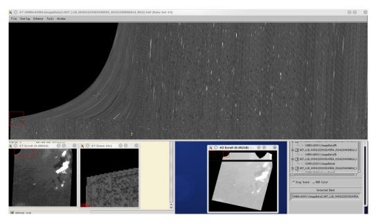
Figure 6-4. Top Warping AST\_L1B Which Fails AST\_L1T PGE.
