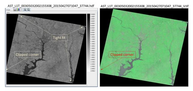
Figure 6-2. Clipped Corner for VNIR-only AST\_L1T HDF and \_V.TIF.
