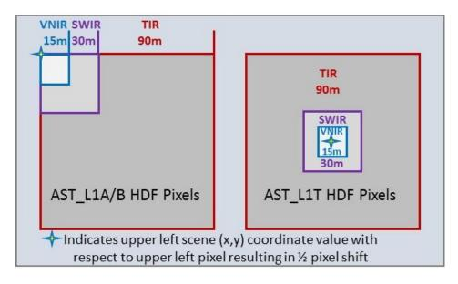
Figure 2-3. Pixel Centering for AST\_L1A/B and AST\_L1T Bands.
