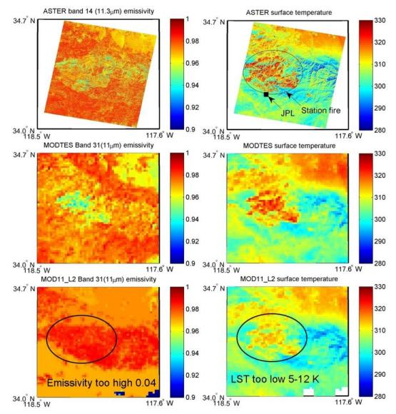
Figure 17. Emissivity images (left) and surface temperature images (right) for ASTER (top), MODIS TES (MODTES) (center) and MODIS SW (MOD11\_L2) (bottom) products over the Station Fire burn scar just north of Pasadena, CA. Location of JPL in Pasadena and burn scar area indicated at top right. MODTES and ASTER results match closely; however, the MOD11\_L2 temperatures are underestimated by as much as 12 K, due to an incorrect emissivity classification.
