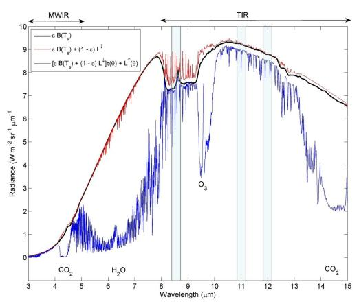
Figure 2. Radiance simulations of the surface-emitted radiance, surface-emitted and reflected radiance, and at-sensor radiance using the MODTRAN 5.2 radiative transfer code, US Standard Atmosphere, quartz emissivity spectrum, surface temperature = 300 K, and viewing angle set to nadir. Vertical bars show placements of the MODIS TIR bands 29 (8.55  $\mu$ m), 31 (11  $\mu$ m), and 32 (12  $\mu$ m).
