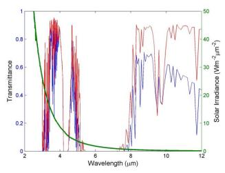
Figure 1. Simulated atmospheric transmittance for a US Standard Atmosphere (red) and tropical atmosphere (blue) in the 3–12 μm region. Also shown is the solar irradiance contribution W/m<sup>2</sup>/μm<sup>2</sup>.
