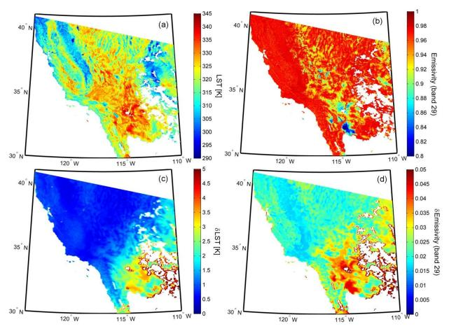
Figure 21. MODIS TES retrievals including WVS correction over the southwestern United States on 7 August 2004: (a) (top left) LST, (b) (top right) emissivity for band 29 (8.55  $\mu$ m), (c) (bottom left) LST uncertainty, and (d) (bottom right) emissivity uncertainty for band 29 (8.55  $\mu$ m). White areas over land indicate areas of cloud that have been masked out using the MOD35 cloud mask product.
