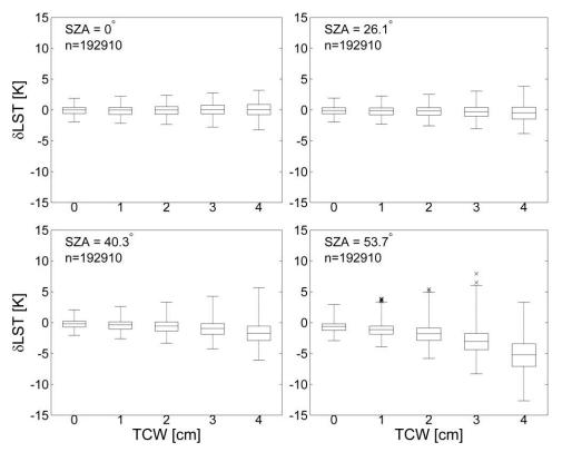
Figure 20. MODIS LST uncertainties using the TES algorithm versus TCW for four viewing Gaussian angles of 0°, 26.1°, 40.3°, and 53.7°. The value *n* represents the number of data points used for a specific land surface type, in this case bare surfaces (rocks, soils, sands).
