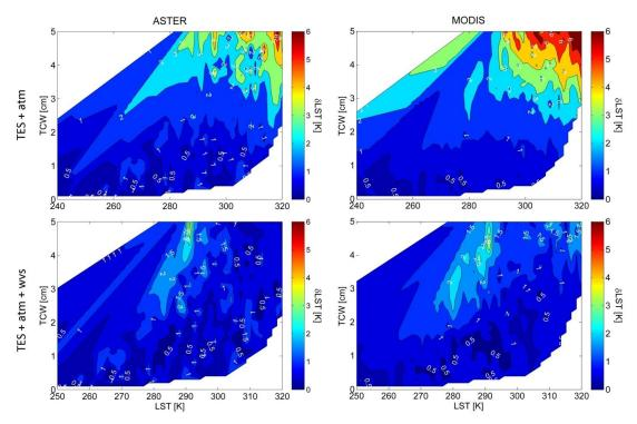
Figure 10. ASTER (left panels) and MODIS (right panels) LST uncertainty distributions plotted versus TCW and simulated LST for all end-member surface types (graybody, soils, sands, and rocks), for the TES algorithm including atmospheric error (TES+atm) and with the WVS method applied (TES+atm+wvs).
