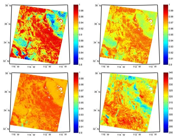
Figure 13. Clockwise from top left: MODIS cutouts of land surface emissivity for band 29 (8.55  $\mu$ m); band 31 (11  $\mu$ m), band 32 emissivity (12  $\mu$ m), and LST output from the TES algorithm over the Imperial Valley, southeastern California on 29 August 2004.
