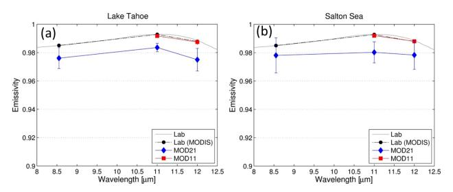
Figure 22. Figures showing the Emissivity retrievals for the MODIS Aqua MYD21 products over two water sites using data collected for three years of data for Lake Tahoe (2003-2005) and Salton Sea (2008-2010). Lab data, Lab data convolved with MODIS bands and the MOD11 bands 31 and 32 are also shown for comparison.
