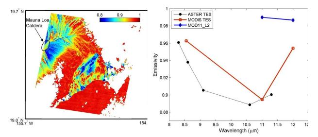
Figure 18. (left) ASTER band 12 (9.1 μm) emissivity image over Mauna Loa caldera, Hawaii on 5 June 2000, and (right) emissivity spectra from ASTER, MODTES, and MOD11 emissivity classification. While ASTER and MODTES agree closely, MOD11 emissivities are too high, resulting in large LST discrepancies between MODTES and MOD1 (12 K) due to misclassification in bands 31 (11 μm) and 32 (12 μm).
