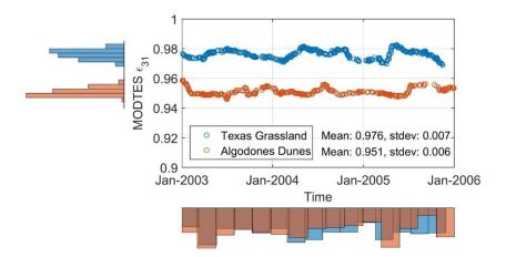
Figure 28. MYD21 Emissivity retrievals for band 31 at the two sites show small fluctuations within the error range of 1% from the mean values. The histograms on the margins show a consistently high density of the data around the mean for each of the sites.
