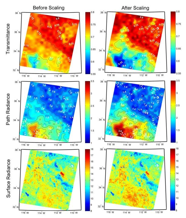
Figure 5. Comparisons between the atmospheric transmittance (top), path radiance (W/m<sup>2</sup>/ $\mu$ m<sup>-1</sup>) (middle), and computed surface radiance (W/m<sup>2</sup>/ $\mu$ m<sup>-1</sup>) (bottom), before and after applying the WVS scaling factor  $\gamma$  to a MODIS scene cutout shown in Figure 5. Results are shown for MODIS band 29 (8.55  $\mu$ m).
