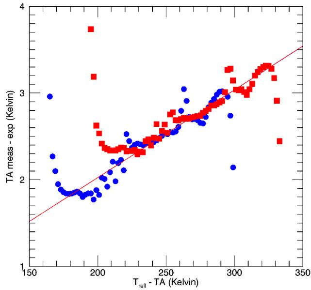
Figure 4: Regression of  $T_A$  measured minus expected versus binned  $T_{refl} - T_A$ .  $T_{refl}$  is the physical temperature of the antenna (from the JPL thermal model).  $T_A$  is the radiometric antenna temperature. Blue: V-pol. Red: H-pol. The slope of the linear fits is the reflector emissivity. The bin population (not shown) is very small at the lower and upper end of the x-axis interval, which causes the outliers.
