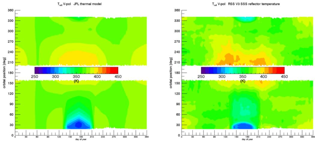
Figure 5: Physical temperature  $T_{refl}$  of the reflector. Left: JPL thermal model that is used in the SMAP L1B files (Piepmeier et al. 2018). Right: Reflector temperature in the RSS SMAP Version 3 release after the empirical adjustment  $\Delta T_{refl}$  has been added.
