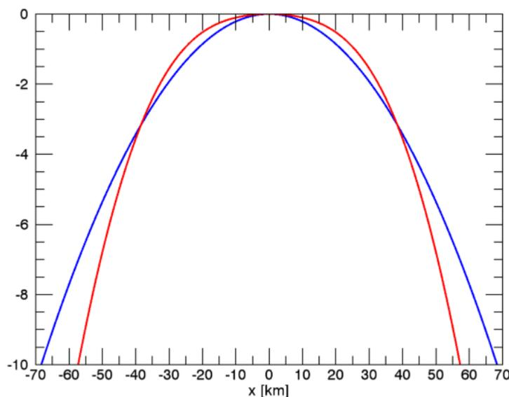
Figure 1: 1-dimensional cross section of spatial response functions (in dB): Blue: Gaussian gain pattern with half-power footprint diameter of 75 km. Red: Average of 3 Gaussian gain patterns whose half-power footprint diameters are 40 km each and who are centered at 0, +25 km, -25 km.
