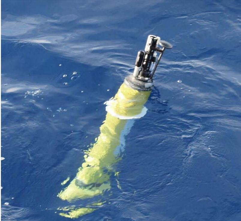
Figure 3.98. PAL sensor on an Argo float ([Riser et al. 2019](#)). The PAL hydrophone is the disk-shaped extension at the top.
