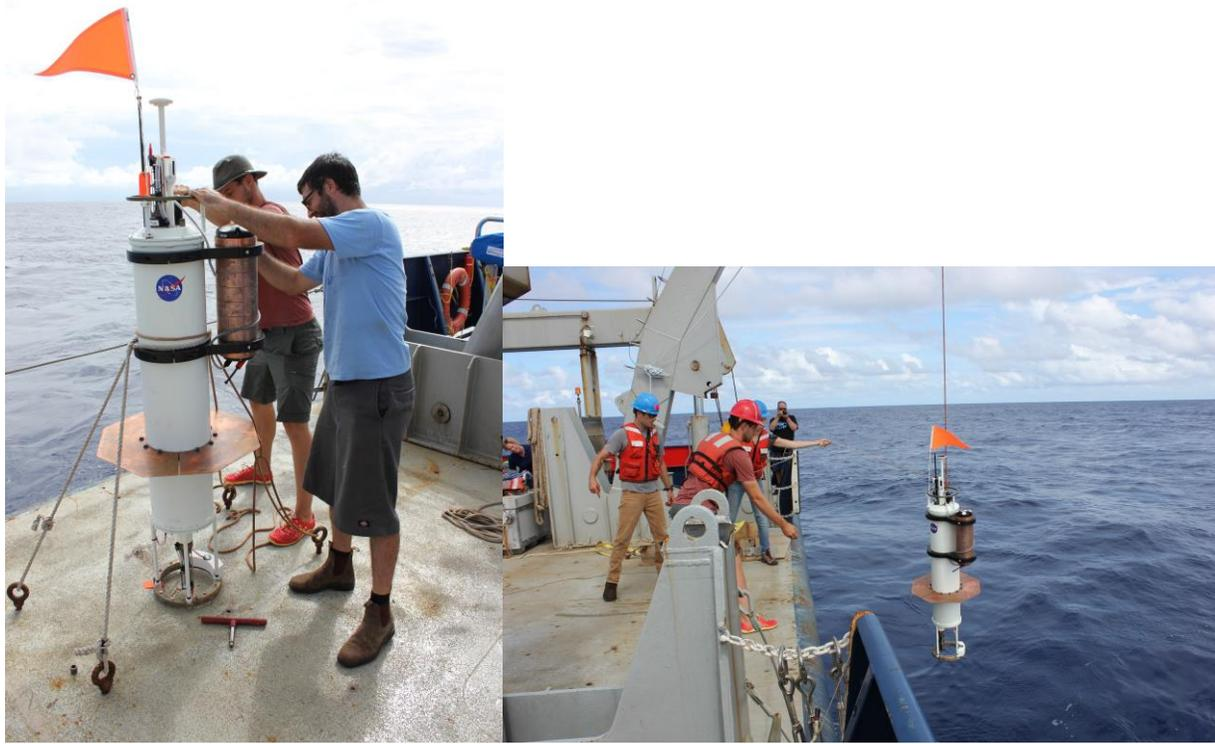
Figure 3.83. Mixed-layer float being deployed from the Revelle. Photo courtesy of A. Jessup.
