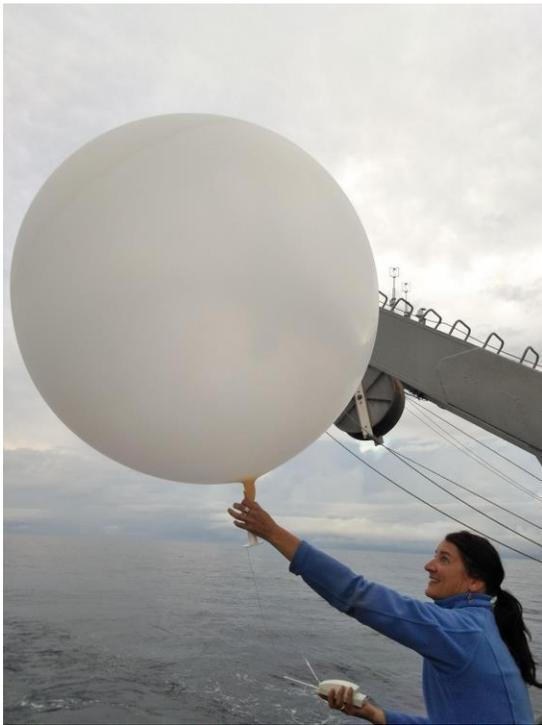
Figure 3.32. A rawinsonde being released off the aft deck of the Revelle during cruise 2. Image courtesy of Ben Greenwood.
