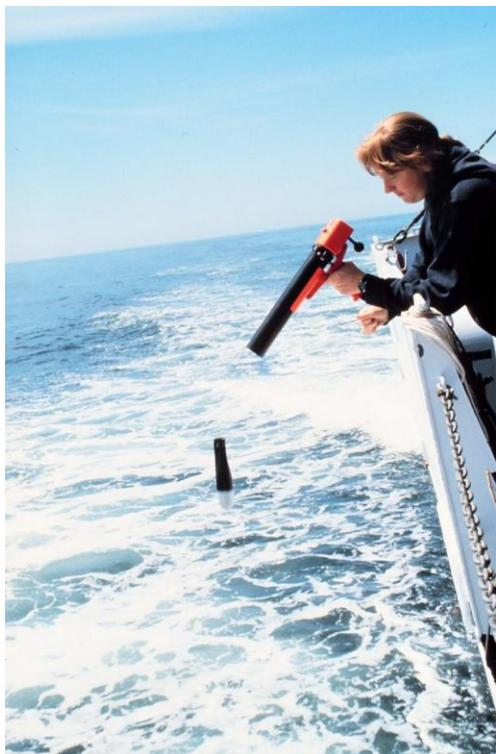
Figure 3.18. Expendable bathythermograph (XBT) being launched from a vessel ([Wikimedia Commons 2019](#)).
