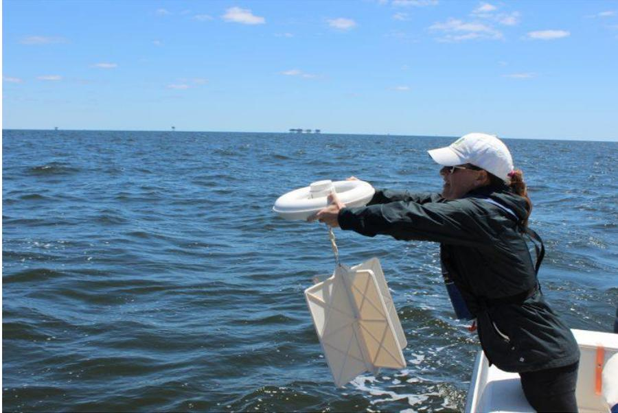
Figure 3.67. A CARTHE drifter being deployed ([CARTHE 2016](#)).
