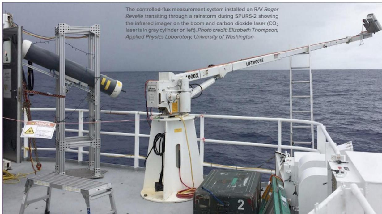
Figure 3.37. The controlled-flux measurement system installed on the Revelle. Photo taken from Asher et al. (2019).
