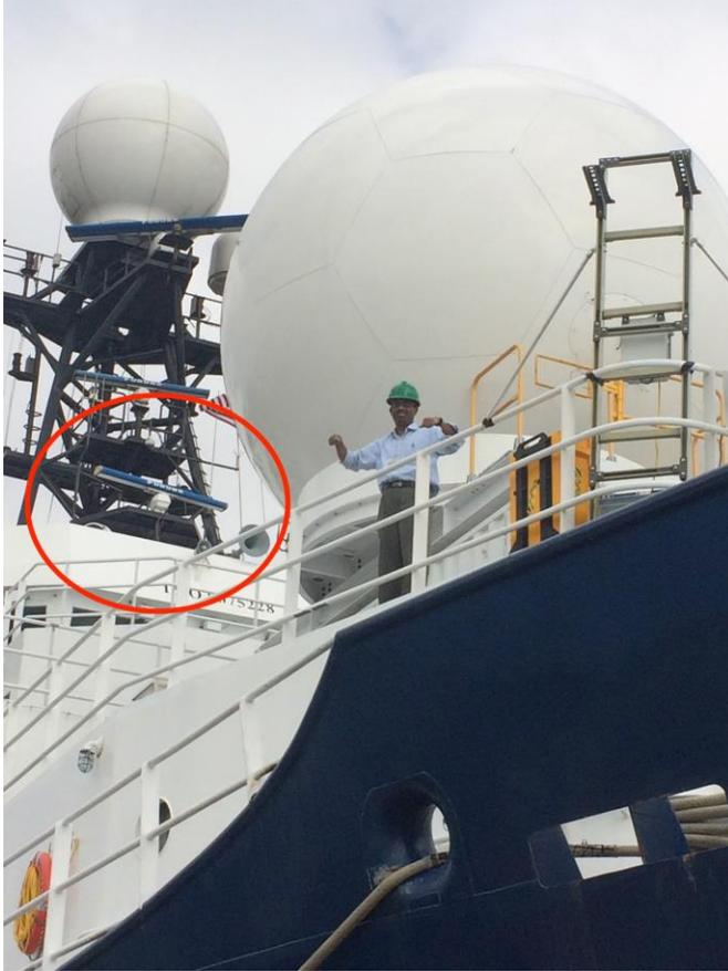
Figure 3.45. The mast of the Revelle, and the SEA-POL radar. The X-band radar is circled. Image courtesy of E. Thompson.
