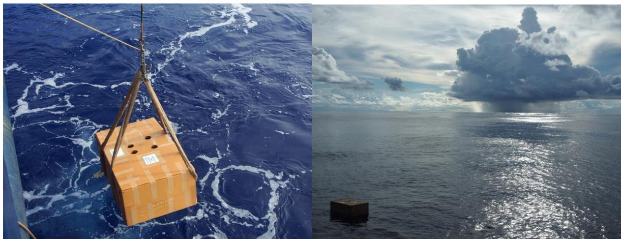
Figure 3.56. SVP drifters being deployed from the Revelle. Photo courtesy of Audrey Hasson.
