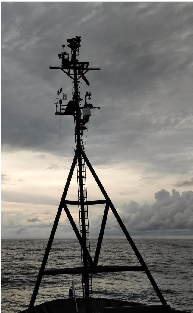
Figure 3.28. Meteorological instruments on a mast mounted on the bow of the Revelle on cruise 2. Photo courtesy of Ben Greenwood.
