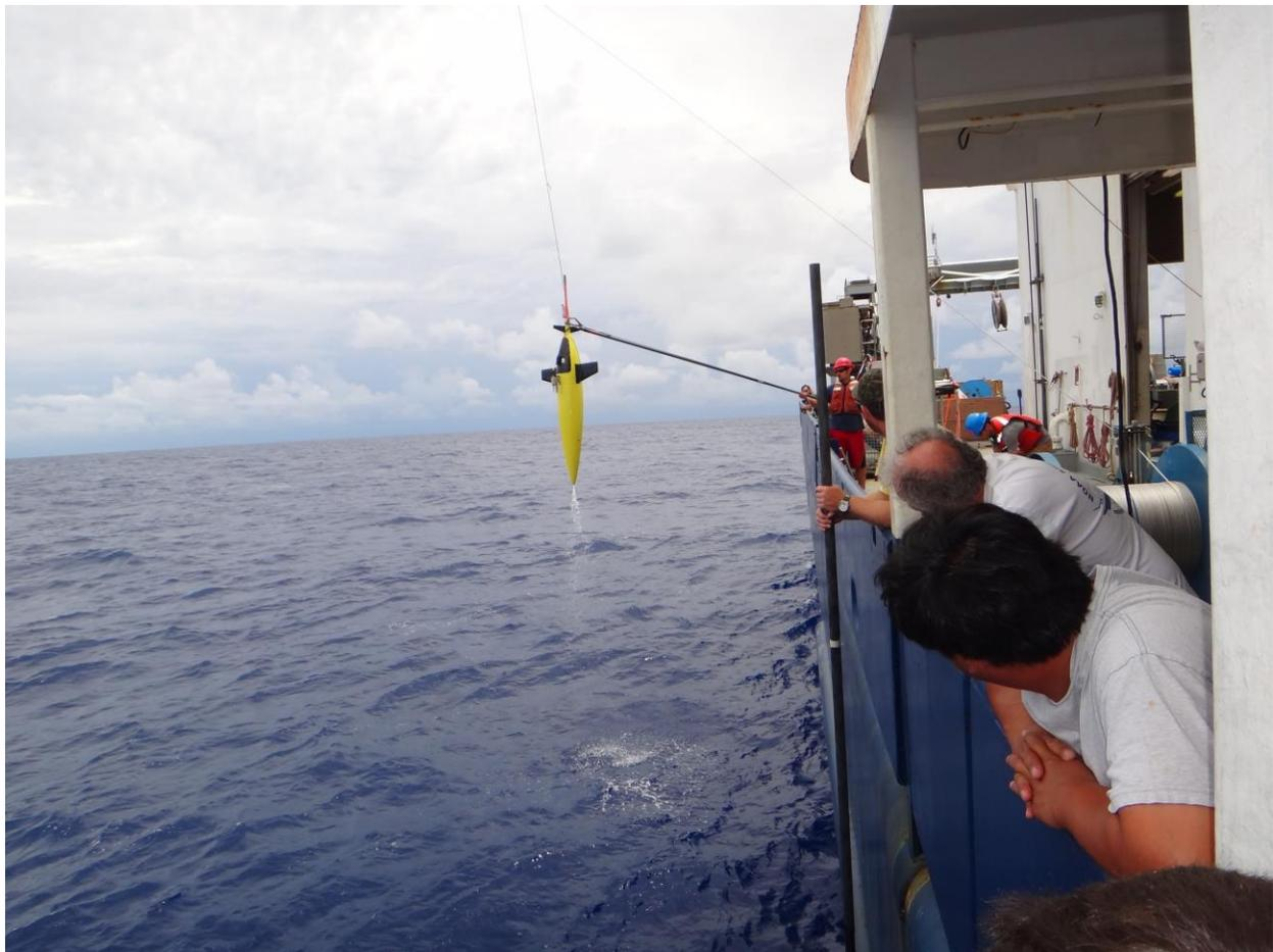
Figure 3.93. Seaglider being deployed from the Revelle.
