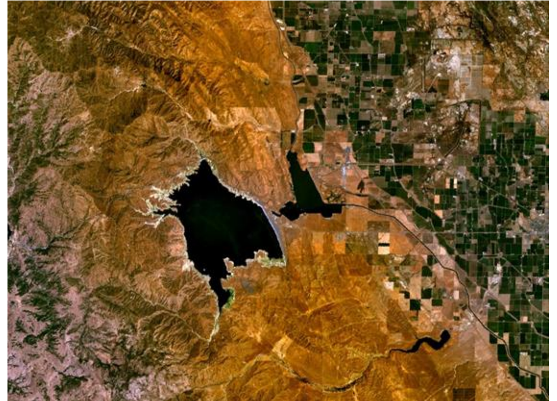
Landsat 7 image of the San Luis Reservoir in Merced County, California. The reservoir stores water taken from the San Joaquin-Sacramento River Delta and is an example of an off-stream reservoir. Credit: NASA
