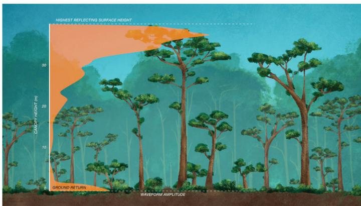
Artist's rendering of how the GEDI LIDAR samples forest canopy height and structure. GEDI has the highest resolution and densest sampling of any LIDAR ever put in orbit. Screenshot from a video produced by NASA's Scientific Visualization Studio and available at <https://svs.gsfc.nasa.gov/13090>.
