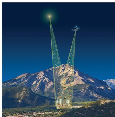
*Sunlight rays entering the OCO-3 instrument pass through the atmosphere twice: once as they travel from the Sun to Earth and then again as they bounce off Earth's surface to the instrument. NASA JPL/Caltech illustration.*
