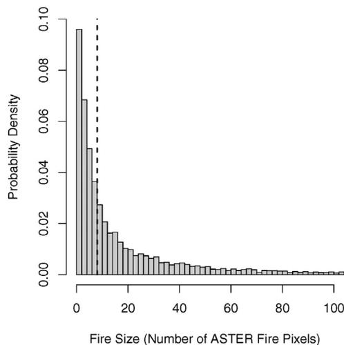
**Fig. 12.** Representative distribution of fire sizes as determined with ASTER, i.e., the number of 30-m ASTER fire pixels within a 1-km MODIS pixel, for the NH Africa region. For clarity, the plot truncates the distribution at just over 100 ASTER fire pixels; in actuality the right tail of the distribution extends well beyond 1000 ASTER fire pixels due to a handful of extreme cases. The dashed vertical line marks the location of the median of the distribution.
