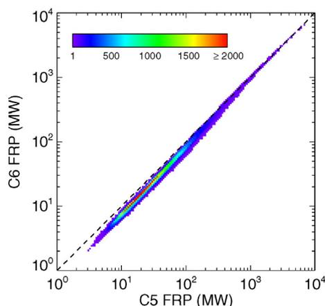
**Fig. 6.** Collection 6 (C6) versus Collection 5 (C5) fire radiative power (FRP) for approximately 240,000 Terra and Aqua MODIS fire pixels detected globally from 1 to 10 August 2005. The color scale indicates the number of points within each element of a  $200 \times 200$  grid that partitions the two-dimensional space bounded by the axes.
