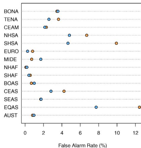
**Fig. 13.** Regional commission error (false alarm) rates for MOD14 Collection 5 (orange dots) and Collection 6 (blue dots). (For interpretation of the references to color in this figure legend, the reader is referred to the web version of this article.)
