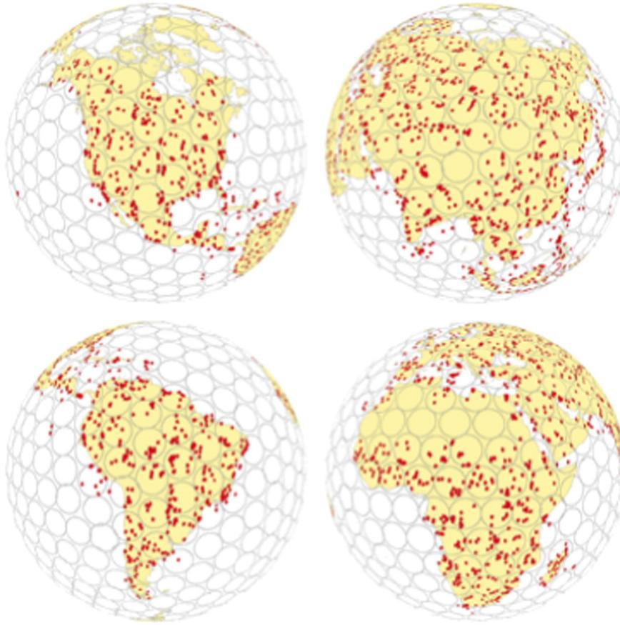
**Fig. 7.** Global equidistant 900 km resolution sampling grid and the distribution of individual  $60 \times 60$  km ASTER reference scenes (red shade) used to validate the near-nadir 1-km Terra MODIS fire product.
