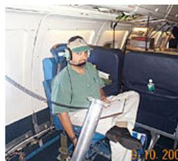
Research scientist Jeff Halverson prepares a dropsonde for release. (Image courtesy of CAMEX-4)
