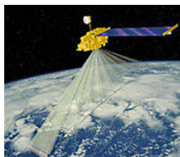
Viewing the sunlit Earth simultaneously at nine widely spaced angles, MISR collects global images with high spatial detail. It captures these images in four colors at every angle.
