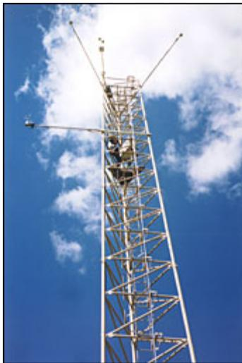
The Skukuza FLUXNET tower in Kruger National Park, South Africa, houses a variety of instruments that measure atmospheric chemistry, humidity, air temperature, soil temperature, and soil water content. (Image courtesy of Bob Cook, Oak Ridge National Laboratory)
