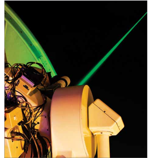
A Satellite Laser Ranging (SLR) Station at Graz Observatory in Austria beams a laser into space, tracking the Environmental Satellite (Envisat). This SLR station acts as the active station, sending off photons, while nearby stations act as passive stations, receiving the Graz photons. (Courtesy H. Wirnsberger)
