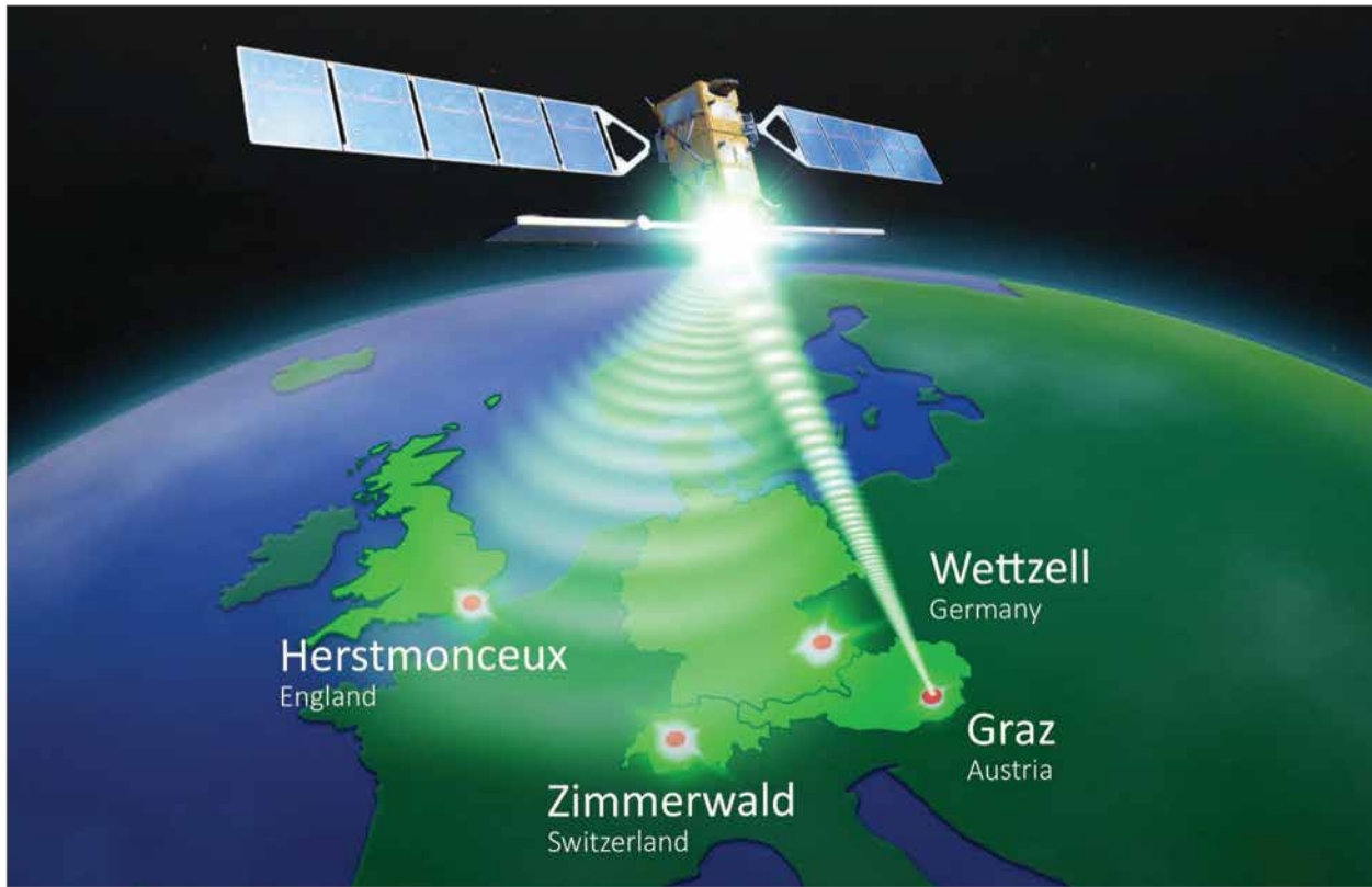
This illustration shows where diffuse photons were picked up by three other passive stations: Zimmerwald, Switzerland; Herstmonceux, England; and Wettzell, Germany. The Satellite Laser Ranging station at Graz, Austria, sent out the initial pulse, rendering it the active station. (Courtesy P. Ruzek, Astronomy Institute University Bern, Switzerland)
