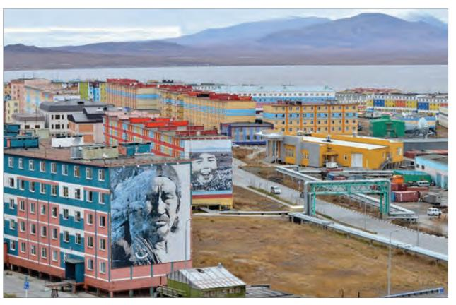
These buildings in Anadyr, Russia, are built on foundation piles to prevent heat from thawing the frozen ground below. (Courtesy US Consulate Vladivostok)
