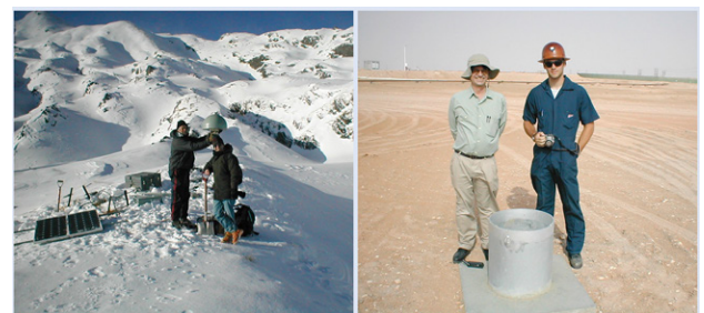
Dr. Herring uses GPS in studies around the world. Left image: Dr. Herring (on right) and a colleague in the New Zealand Southern Alps using GPS to measure vertical uplift across Southern New Zealand (the GPS receiver is the gray helmet-looking object above Dr. Herring). Right image: Dr. Herring (on left) and a colleague in Oman using GPS to measure subsidence and horizontal motions due to oil and gas extraction. The canister in front of Dr. Herring protects the GPS antenna, which is inside. Images courtesy of Dr. Herring.
