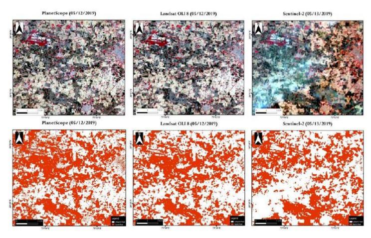
Visible imagery and burnt area extent derived from PlanetScope (left column), Landsat (middle column), and Sentinel-2 (right column) over Barnala, Punjab, India. Using a single date 90% cloud free imagery, PlanetScope was able to detect 5% percent more burnt area than Landsat and 9% more than the Sentinel.
