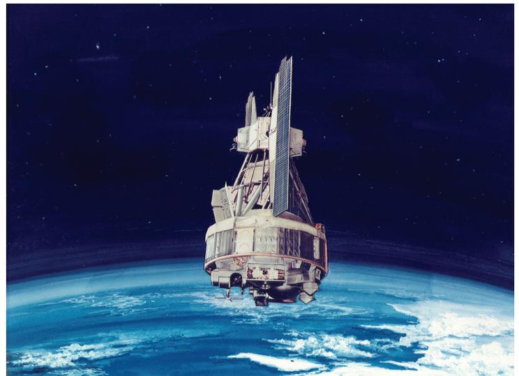
*Nimbus I launched on 28 Aug. 1964 and operated until 22 Sept. 1964. Along with the HRIR instrument, the spacecraft also carried an advanced vidicon camera system (AVCS) for recording and storing remote cloud cover images and an automatic picture transmission (APT) camera for providing real-time cloud cover pictures. NASA graphic*
