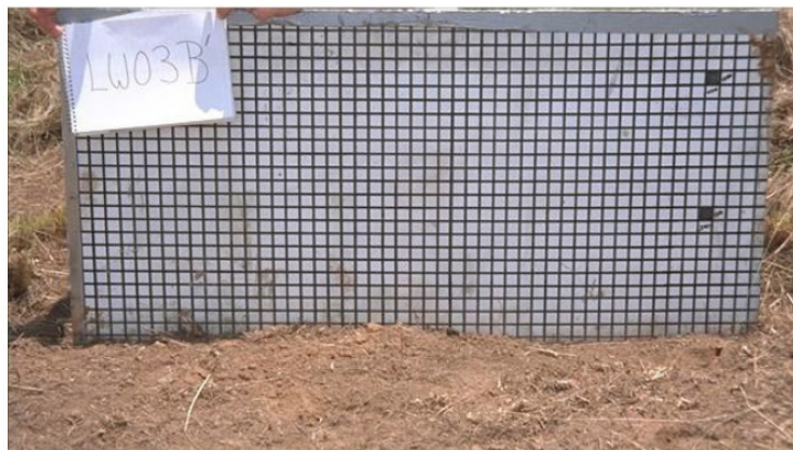
Assessing surface roughness using a grid board. The card in the upper left corner of the board is the site ID. Image from the SMAPVEX16 Iowa Experiment Plan.
