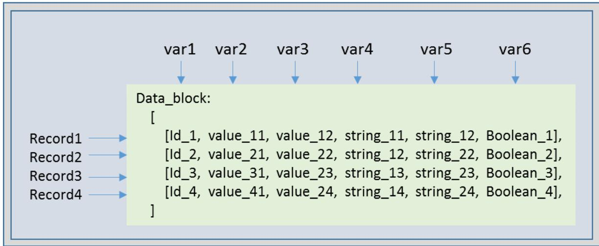
**Figure 2. Standard data-block structure diagram for two-dimension data records, row for each record and column for each variable.**
