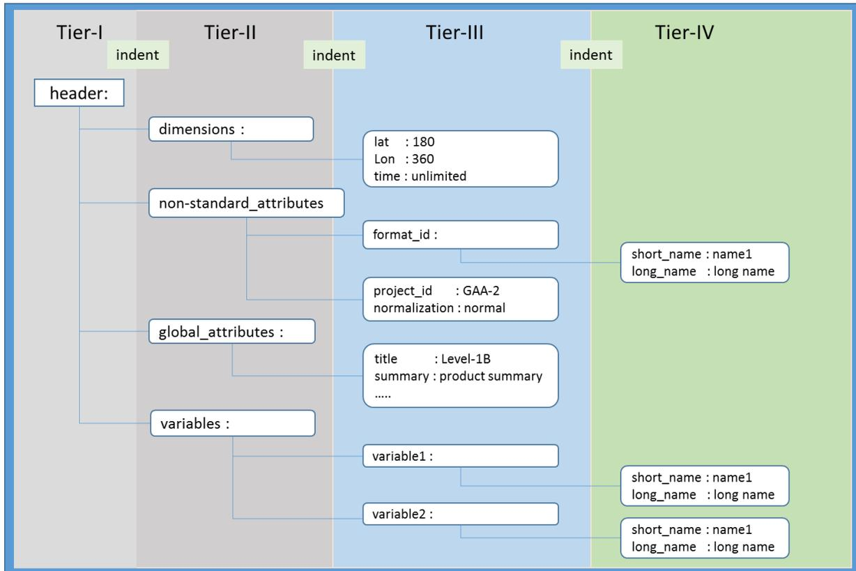
Figure 1, YAML header structure scheme, which contains four major sections (*dimensions*, *non-standard\_attributes*, *global\_attribute*, and *variables*), and four layers of nested sub-structures (denoted by four Tiers).
