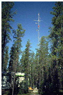
Measurements of the boreal forest are taken through a flux tower. (Image courtesy of The BOREAS Project)
