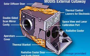
**Description:** Medium-resolution, multi-spectral, cross-track scanning radiometer
