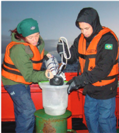
Dr. Lange (left) and Dr. Rafael Araujo (right, Technical University of Denmark, Kongens Lyngby (DTU)) collecting surface water samples with a Van Dorn bottle on board the Brazilian Research Ship Ary Rongel at the Bransfield Strait, Antarctic Peninsula, in February 2010. Image courtesy of Dr. Lange.
