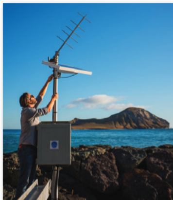
Dr. Philip Thompson checks a tide gauge solar panel mount on Makai Pier, Oahu, Hawai'i. Image by Elyse Butler.
